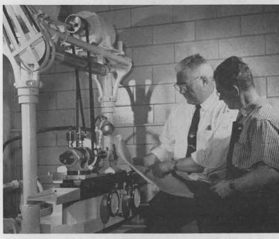
UNIVERSAL CYLINDER GRINDER has been operated by Rex Rozelle in forming this experimental mandrel for air bearing application studies. Supervisor C. C. Paschal checks dimensions.
